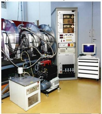
In the field of semiconductor research atomic particle sources are needed with defined particle speeds and thus energy levels (E=mc2). These sources are mounted next to atomic research reactors, which produce a wide spectrum of sub- atomic particles of different masses and energy levels.A mechanical chopper system is used to select particles within a narrow energy band, by allowing only those particles to pass, which are travelling at a very closely defined speed.
